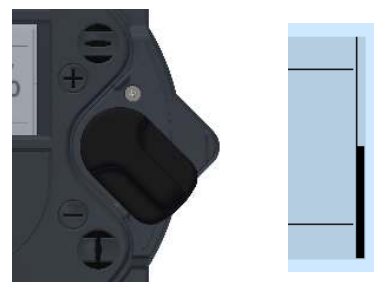
Figure 38: Full switch flip (it will jump to the end of the menu)
